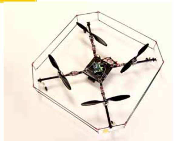
Quadrotor agile autonomous aircraft designed by E. Stingu for urban and cluttered environments
